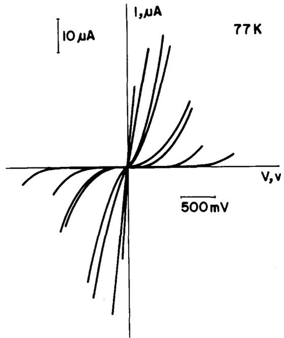
Fig. 2.  $I-V$  characteristics of sample with disordered antidot lattice at various maximum voltage.
